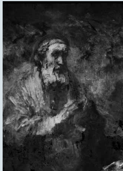
Pb L radiation (high energy - white pigment)
