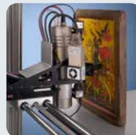
Measurement head with SD detector
