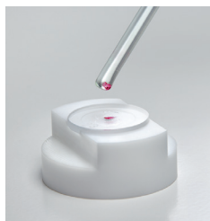
3. Pipette 5 to 20 \mu l on carrier
