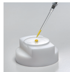
4. Pipette 5 to 20 \mu l on carrier
