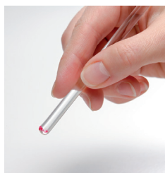
2. Pick-up some particles with (glass) rod
