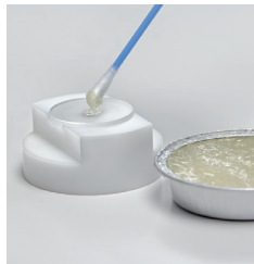
1. Dab vacuum grease on carrier
