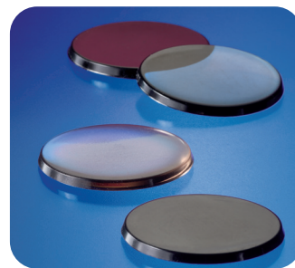
Figure 3: Fused bead samples for XRF analysis
