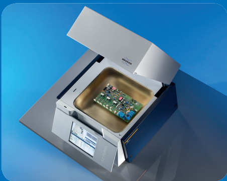
Figure 4: The S2 PUMA Carousel's sample chamber can hold microcircuits in one piece
