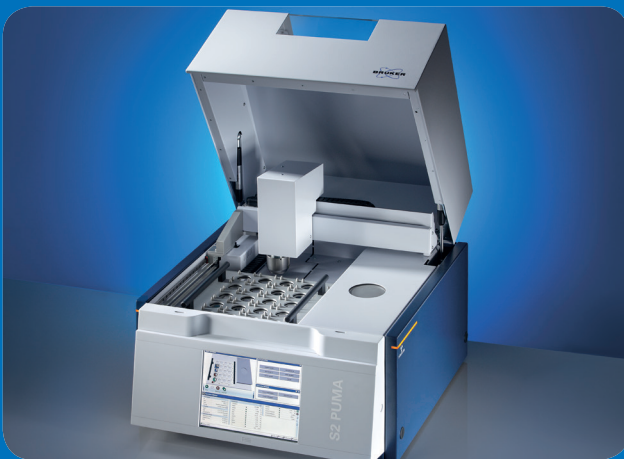
Figure 3: The S2 PUMA XY Autochanger – ideal for applications with high-sample throughput requirements.
