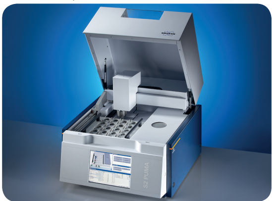
Figure 2: The S2 PUMA XY Autochanger guarantees high sample throughput
