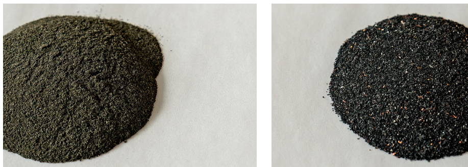
Figure 2 Typical black mass powder samples. Left: Homogeneous sample, ready for immediate analysis as powder or pressed pellet. Right: Coarser, rather heterogeneous sample containing, e.g., Cu particles.
