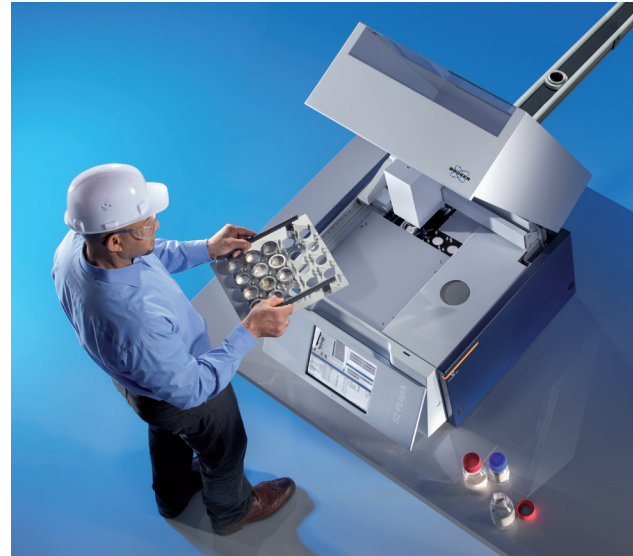
Figure 2: S6 JAGUAR – Ready for Automated Quality Control of Cement Products
