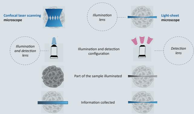
**Figure 2.** Comparison of confocal laser-scanning and light-sheet fluorescence microscopy.
