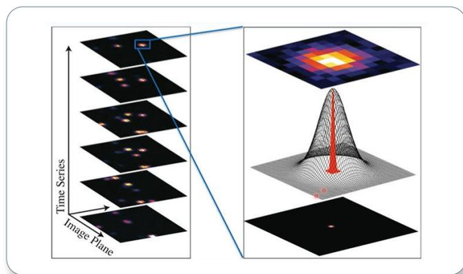
Figure 2. Image acquisitions of single molecules over time with SMLM. Each molecule is imaged stochastically within an imaging plane over time. The point spread function data are collected and used to localize the center of each individual molecule.
