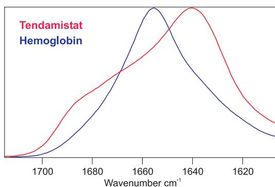
Figure 1A: The amide I band of the IR spectrum of a protein reflects its secondary structure. Here, IR spectra of Hemoglobin and Tendamistat are shown. The Hemoglobin amide I band has a position (~1652 cm<sup>-1</sup>) and shape clearly indicative of a protein with a high  $\alpha$ -helical content. The Tendamistat amide I band is characteristic (broad peak at ~1635 cm<sup>-1</sup>) of a protein with a high  $\beta$ -sheet content.
