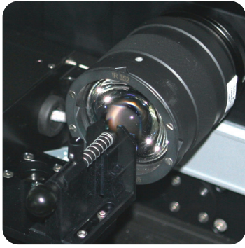
PL II sample compartment with NIR/VIS objective and standard sample stage.
