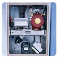
The pre-aligned dual DigiTect™ detectors allow accurate user exchange.
