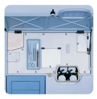
Beamsplitters and sources are easy to exchange and stored inside the optics bench.
