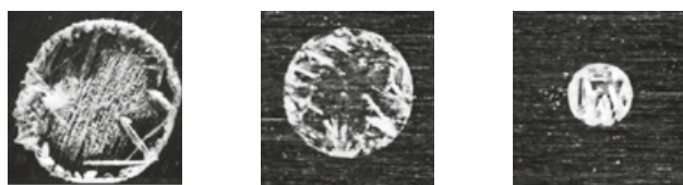
Depending on the sample type, a larger or smaller diameter AnchorChip target may be selected. The examples above demonstrate crystallization of DHB to a standard stainless steel, 800 \mu\text{m} and 2000 \mu\text{m} AnchorChip targets (left to right).
