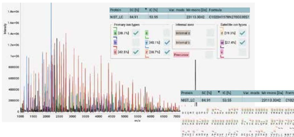
Sequence verification of NIST mAb light chain by MALDI top-down sequencing (MALDI-TDS). Simple and robust sequence readout that does not require charge deconvolution. Matching MALDI-TDS data against a target protein sequence using Bruker OmniScape software requires only few mouseclicks. Confident sequence confirmation with a short time to result enables instant decision making.
