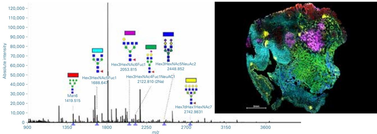
Mean spectrum of the entire N-glycan MALDI Imaging dataset from a colorectal cancer section and multichannel ion image showing the distribution of the indicated peaks (blue triangles under the x-axis).
