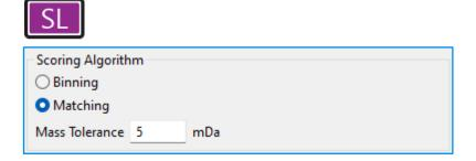
The Spectral Library annotation tool uses cosine scores to assess matches between measured and reference spectra. Now a mass tolerance-based matching algorithm is used to associate the respective signals from both spectra and replaces the former binning algorithm. This change results in a more reliable and intuitive association of mass signals, leading to more representative scoring.
