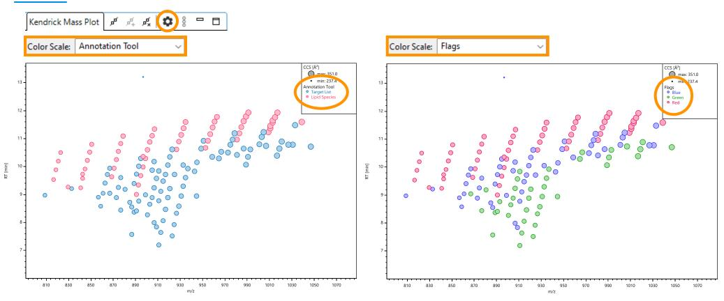
The new Color Scale options in the Kendrick Mass Plot / Survey View enable users to highlight features based on the annotation tools used or their first flag color. In the examples above, the left image shows TG lipids annotated with the Lipid Species tool, while further oxidized TGs were identified using a dedicated Target List. In the right image, red, blue, and green flags indicate TGs that are unoxidized, oxidized once, and oxidized twice, respectively.
