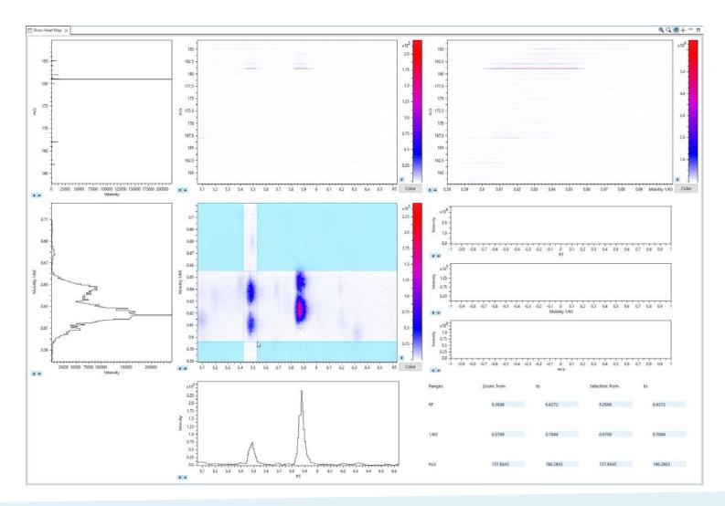
To get clear EIC, EIM, and average MS spectra for the two signals in range RT 5.45 – 5.25 min and 1/K<sub>0</sub> 0.595-0.655 [Vs/cm<sup>2</sup>] select box selection mode and drag a box with the mouse in region interest
