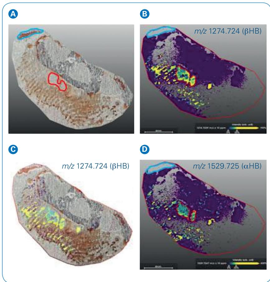
Figure 2. MALDI MSI of a human blood fingermark of 4 years of age stored in uncontrolled ambient conditions. (A) optical image; (B) and (D) MALDI MS image of the HB ions at  $m/z$  1274.724 ( $\beta$ HB) and 1529.725 ( $\alpha$ HB) respectively, measured with a 10 ppm mass accuracy. (C) Overlay of the image at  $m/z$  1274.724 with the optical image. Blue and red framed highlight: regions of the mark where blood is visible or not visible respectively, on the optical image.
