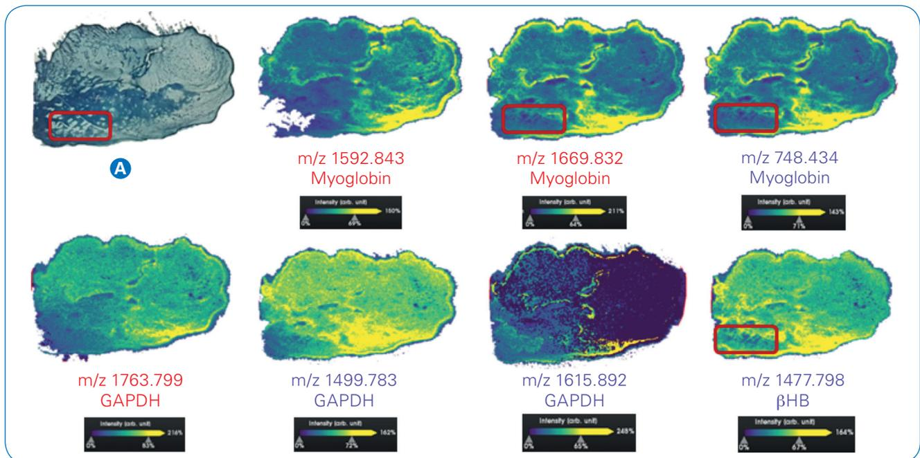
Figure 6. Many ion signals were recovered indicating the presence of blood through Haemoglobin, Myoglobin and GAPDH. A selection of such images is presented here. **A** shows the optical image of the AB-1 enhanced bovine blood mark. The red rectangle indicates the presence of ridge flow in both the optical image and some of the MS images. The  $m/z$  values in red indicate the proteotypic bovine blood peptide biomarkers within the system investigated by Kennedy et al. [5].
