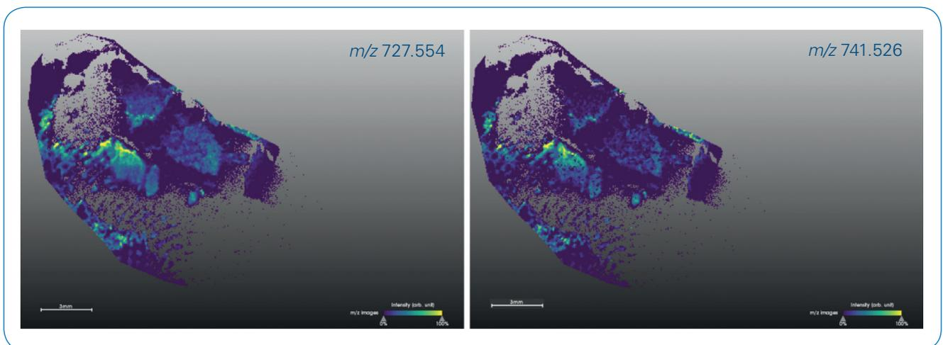
Figure 4. MALDI MS images of lipids at  $m/z$  727.554 and 741.526 in a human blood fingermark. These ion signals show additional ridge coverage with respect to the blood specific protein-deriving peptides.
