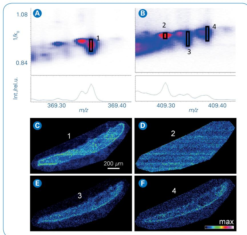
Figure 1. Mobilograms and mass spectra of cholesterol (A, feature 1), sterol  $C_{29}H_{48}O_2$  (B, 3), gorgosterol (B, 4). Also shown is an exemplary feature assigned to matrix-derived chemical noise (B, 2); C, D, E, F show the respective ion images; other matrix- as well as non-sterol derived endogenous analyte signals showed similar compact features. Data were summed across a full section of *Waminoa* but also include areas of matrix-coated substrate next to the tissue.
