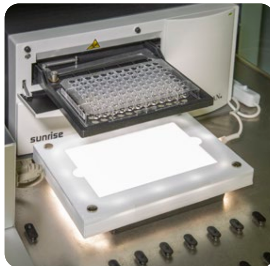
Fig. 3: The SUNRISE Reader allows standardized reading of the MICRONAUT antibiogram and gives proof of adjusted McFarland dilution.
