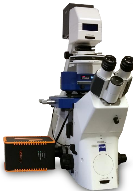
Fig. 1: JPK NanoWizard AFM family integrated with a compact line STEDYCON (Abberior Instruments), on an AxioObserver (Zeiss).
