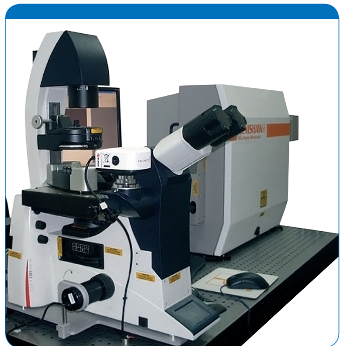
Figure 8. The Bruker BioScope Catalyst AFM shown with a Renishaw inVia Raman microscope.
