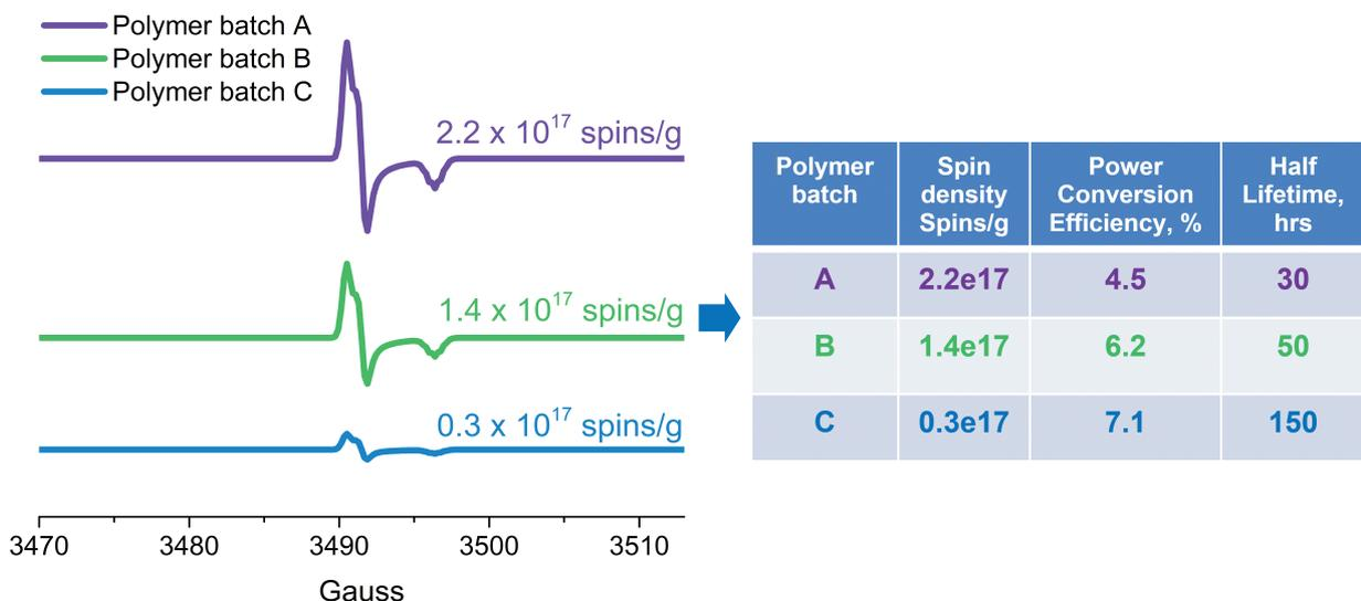
Quantitative EPR analysis of free radical defects presented as spins/g in conjugated polymers (used in solar cells). The number of defects correlates with the solar cell efficiency and stability.
