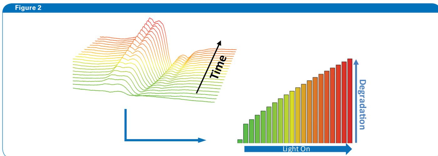
Photodegradation of Nifedipine – time evolution of N-based radical formed in the API and monitored by EPR.
