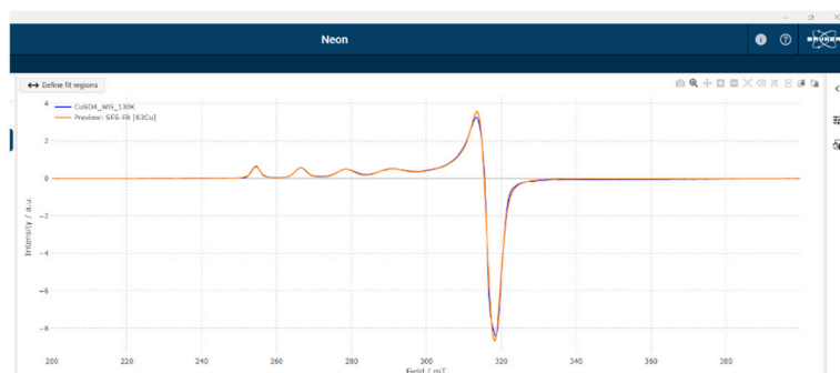
Figure 5: Fitted spectrum of CuSO 4 with g- and A-strain parameters
