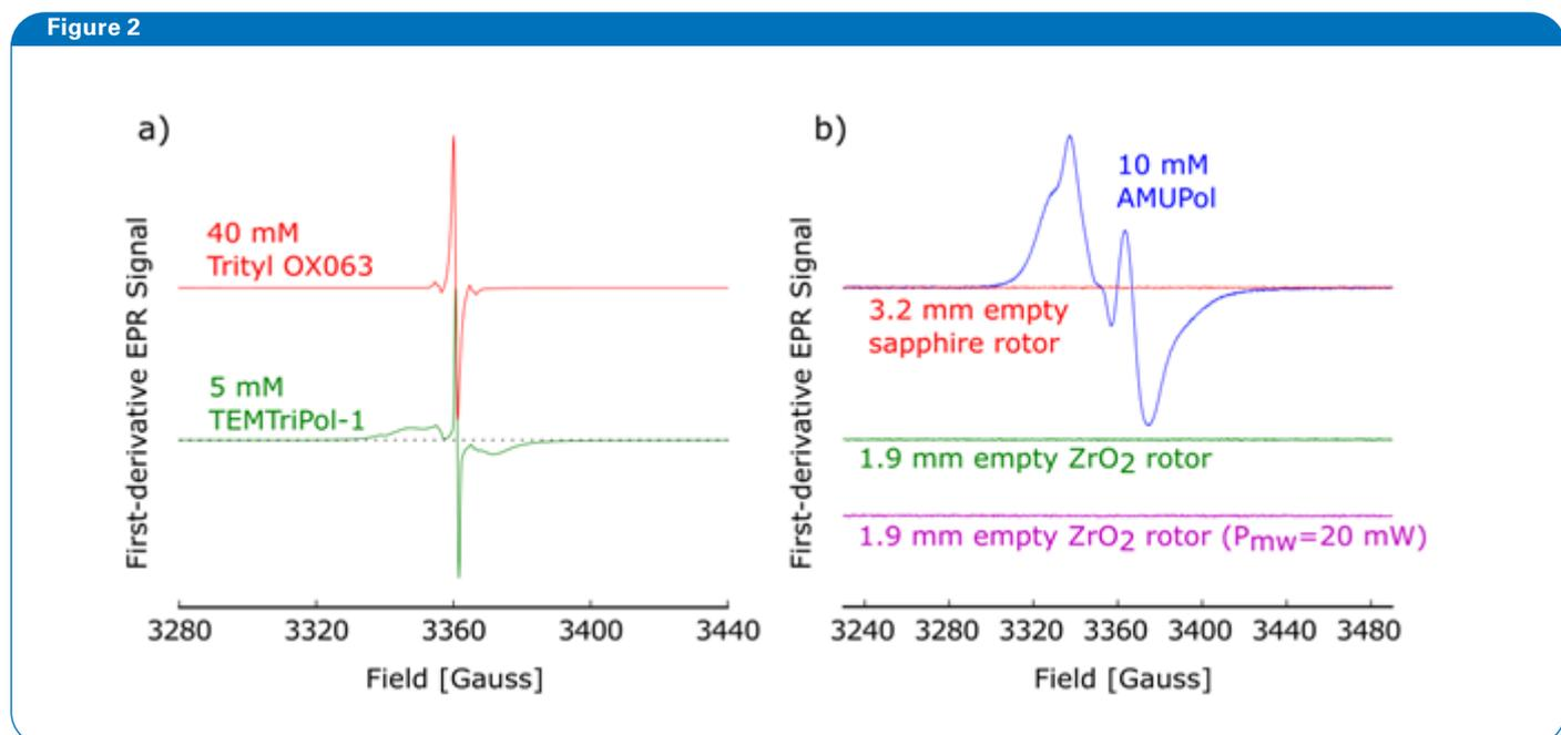
Figure 2: Room-temperature X-band EPR spectra of a) Trityl OX063, TEMTriPol-1 and b) AMUPol radicals acquired on a Bruker Magnetech ESR-5000 spectrometer. At the same measurement parameters, the sapphire and ZrO<sub>2</sub> rotors show no perceivable EPR signals. The microwave power is 1 mW unless specified.
