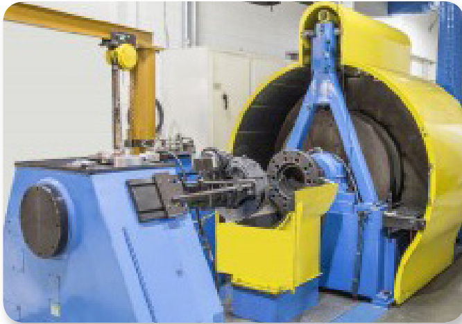
Figure 2. Full-scale brake test protocols/standards are typically conducted on dynamometers. Photo Courtesy of Greening Test Laboratories.
