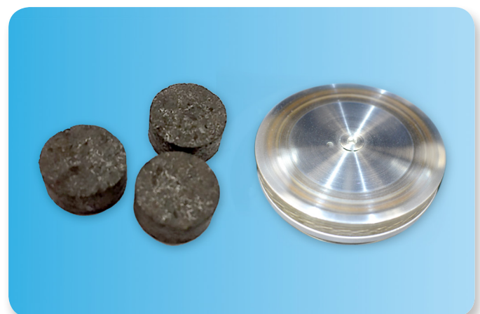
Figure 6. Samples that simulate the brake pad and rotor for testing with the TriboLab Brake Material Screening Tester.
