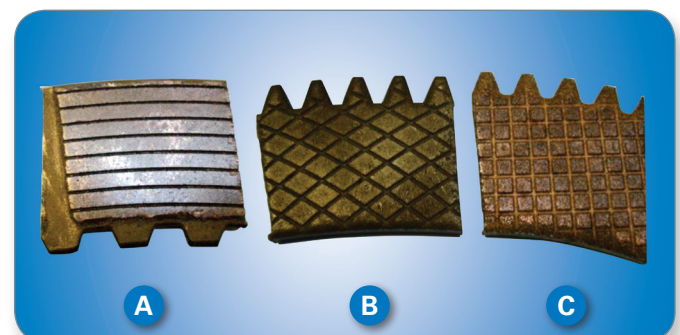
Figure 1. Photos of clutch pieces (a) concentric- (b) diamond- and (c) square-grooved.
