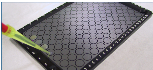
Pipette the samples onto the plate and dry
