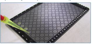
Pipette the samples onto the plate and dry
