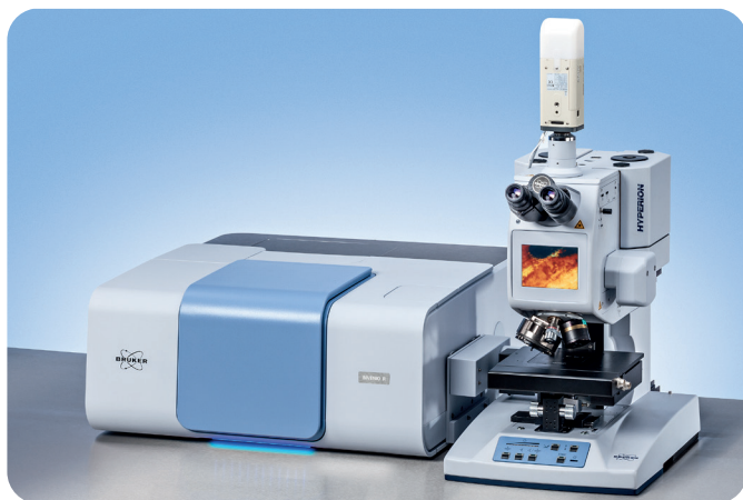
Figure 1: INVENIO with Hyperion microscope.
