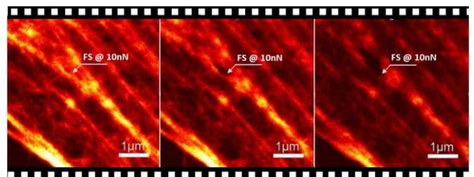
**Fig. 8:** Time series of AFM stimulation-STED measurements. The actin cytoskeleton was labelled with SiR Actin and imaged with an Abberior Instruments Expert Line STED microscope (excitation, 640 nm; STED, 775 nm). The AFM stimulation position is marked with an arrow.
