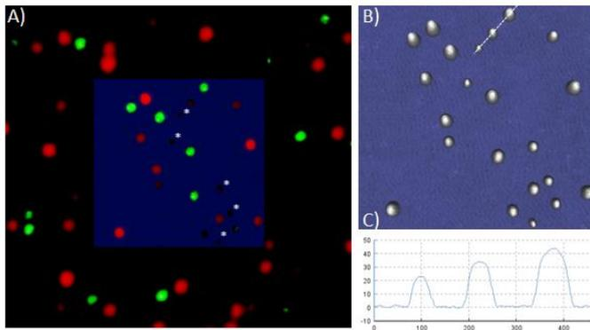
**Fig. 6:** A) Overlay of AFM and STED image. Scan size:  $1\ \mu\text{m} \times 1\ \mu\text{m}$ . Beads measured in AFM that do not correspond to a STED signal are marked with a white star. B) AFM topography image in 3D clearly shows the divergent distribution of bead diameter C) Cross section of three beads.
