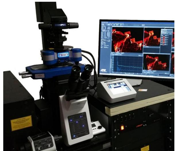
**Fig. 2:** JPK NanoWizard® AFM integrated into an Abberior Instruments Expert Line STED microscope (as an example the NanoWizard® ULTRA Speed is shown).
