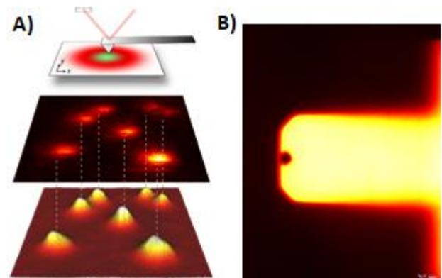
**Fig. 3:** A) STED + AFM principle. STED and AFM images of fluorescence beads as well as correlation of both images are shown [12]. B) Reflection image of Nanoworld USC cantilever.
