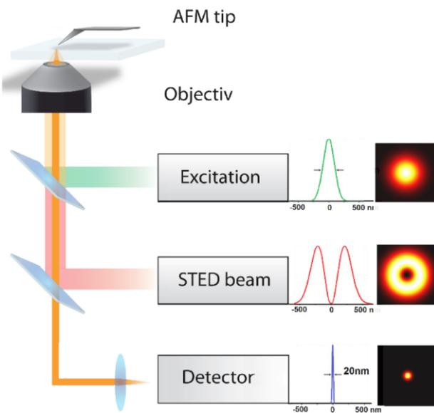
**Fig. 1:** Scheme of an AFM and STED based system showing the major components. The sketch includes the excitation source, the STED beam, the detection unit and the AFM.
