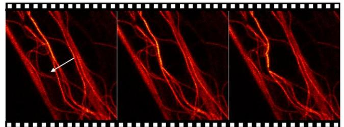
**Fig. 7:** Time series of AFM manipulation-STED measurement. Microtubules labelled with SiR Tubulin and imaged with an Abberior Instruments Expert Line STED microscope (excitation, 640 nm; STED, 775 nm). The AFM manipulation path is marked with an arrow. The manipulation force was set to 5 nN with a velocity of  $1\ \mu\text{m/s}$ .
