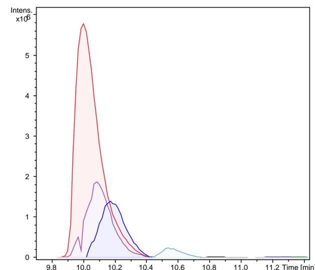
Fig. 6 illustrates the dissect algorithm that is used for compound detection in an LC-MS chromatogram even if the peaks completely overlap. 4 compounds were picked by the dissect software and their corresponding mass spectra seen in Fig. 6 shows distinctly different species.
