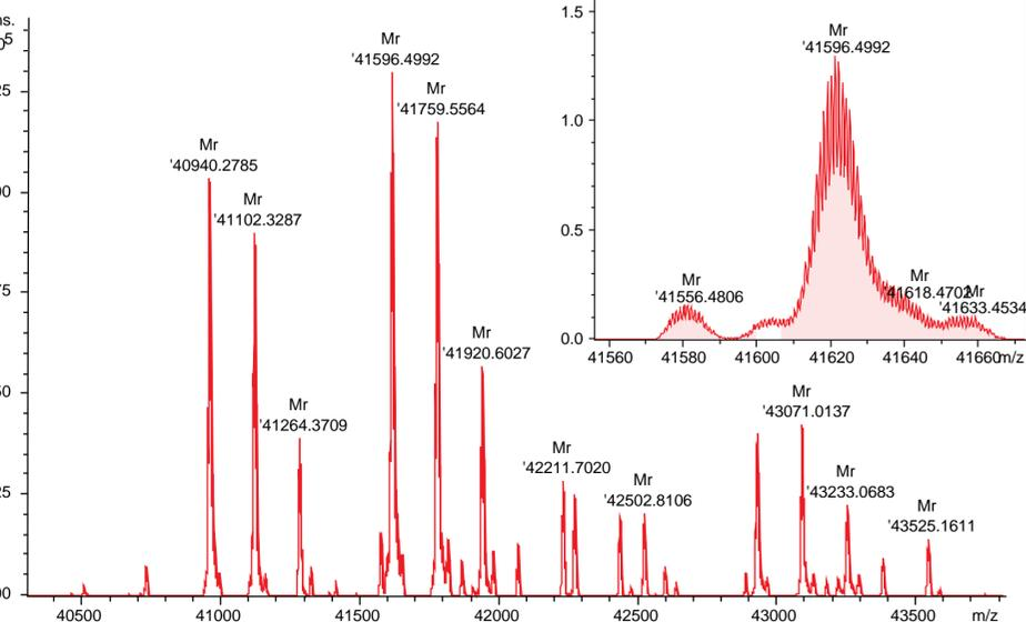
Fig. 1: Fusion protein monomer acquired under denaturing conditions. The high resolving power on the maXis II enables isotopic resolution of the fusion protein as well as maintaining true isotopic pattern™ (TIP) of isotope spacing and intensity under fast HPLC conditions. The SNAP II peak picking algorithm was used to determine the monoisotopic mass of the fusion protein cluster as well as the glycosylation pattern with high mass accuracy.
