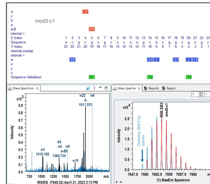
Fig. 2 Auto MSMS analysis of the mod3-c1 variant. The precursor ion isotope pattern (blue) (expected: red) indicates a coeluting species with -1 Da mass difference, the weak MS/MS spectrum was inconclusive.
