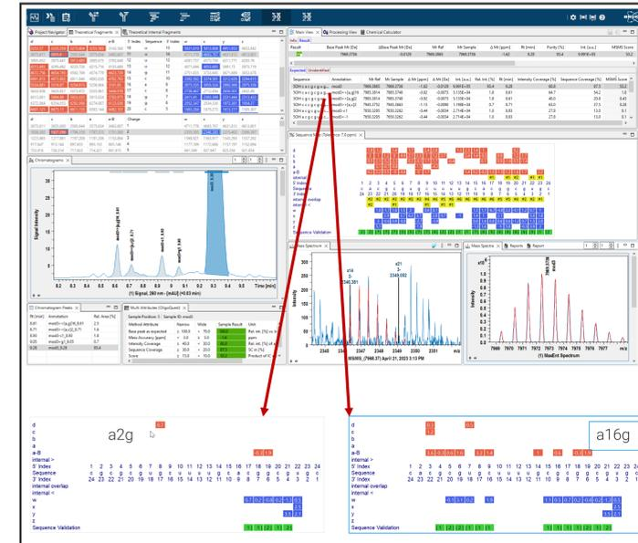
Fig. 1 Top; analysis overview of the FLP mod3, annotated MS and MS/MS peaks overlaid with theoretical isotope patterns. Bottom: Annotation of the variant sequences a2g and a16g
