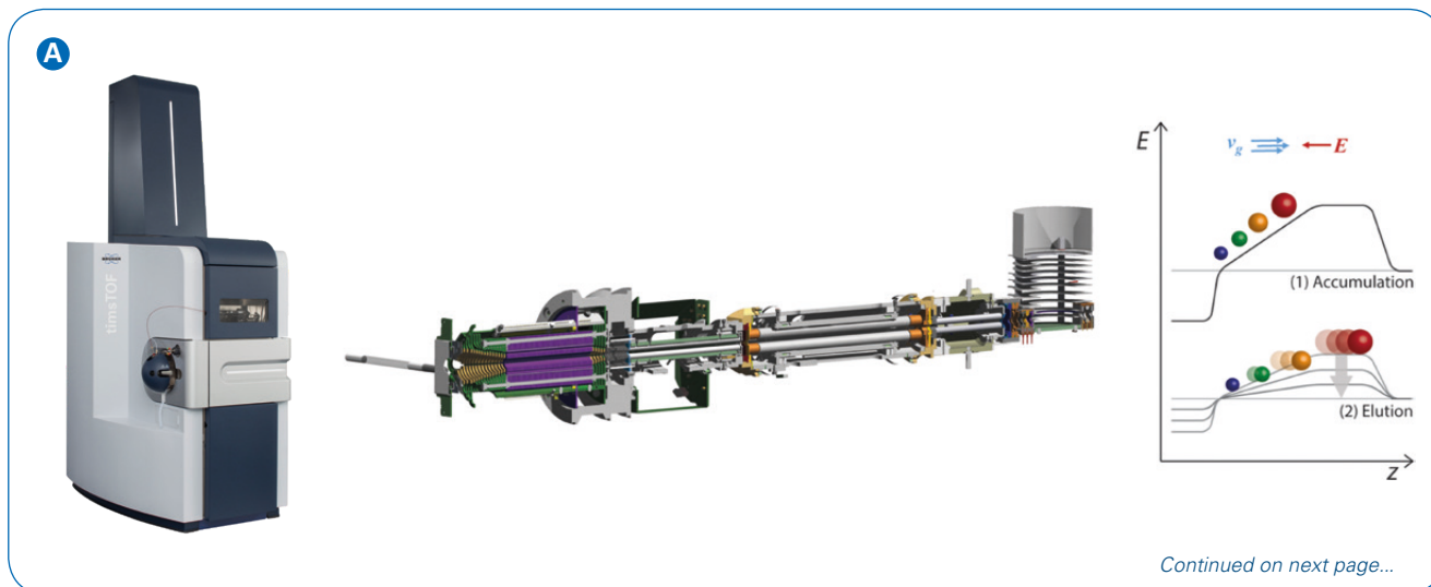
Figure 4: High confidence lipid identification workflow: A real-world example using MetaboScape 4.0. A Lipid extracts from two milk samples were analyzed by LC-MS/MS and LC-TIMS-MS/MS using a timsTOF. Shown are the instrument schematic and TIMS operation from ion accumulation to serial elution, where E represents electrical field and v_g the gas flow. B Box plot of a lipid showing different abundances in two milk lipid extracts detected in ESI positive mode. C Assignment of molecular formula based on accurate mass and true isotopic pattern using SmartFormula™ – C_{38}H_{76}NO_8P . D MS/MS query for ESI positive mode against LipidBlast library returns PC 30:0 as likely candidate. Characteristic head group fragment (184.07 m/z) substantiated assignment as glycerophosphocholine (PC). E SmartFormula3D™ algorithm: Fatty acid chains C14:0 and C16:0 could be assigned based on automatic formulae assignment for characteristic fragment ions in negative mode. F Very low deviation (0.8 %) between measured vs. predicted CCS values (279.7 vs. 277.5) provided further orthogonal confidence for the identification of the target lipid as: PC 14:0_16:0.
