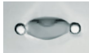
Two beads bound to a red blood cell are used to dynamically stretch it.
