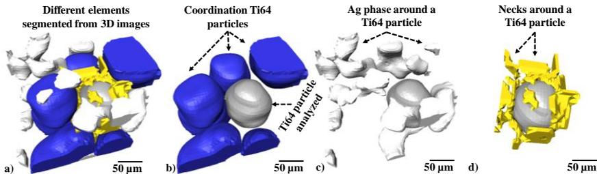
Figure 4. a) 3D rendering of a Ti64 particle surrounded by Ti64 particles in contact with it and necks developed among them and Ag liquid. b) coordination particles around a Ti64 analyzed particles, c) Ag liquid surrounded the analyzed Ti64 particle and d) necks developed during sintering between the contacting Ti64 particles.
