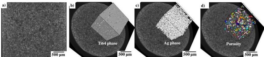
Figure 1. a) 2D virtual slice of transversal section of the Ti64/20Ag composite, b), c) and d) 3D inner volume rendering of the Ti64, Ag and pores phases, respectively.
