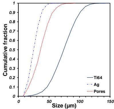
Figure 3. Size distribution of the Ti64, Ag and pore phases.
