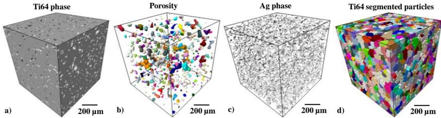
Figure 2. 3D rendering of; a) Ti64, b) Ag and c) pores phases, and d) 3D rendering of the Ti64 particles separated.
