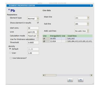
The software provides a variety of options for optimizing methods. These options include different models for deconvolution, selection of used fluorescence (K or L-series, or even change from La to L $\beta$ ).
