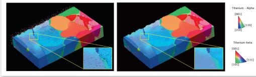
Left: Raw data cube acquired from a TA6V sample. Right: Filtered data cube. Misindexed and isolated voxels can be removed using the "despeckle" filter while linear (Gaussian) and non-linear (Kuwahara and median) filters offer advanced orientation averaging capabilities.
