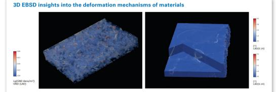
Left: GND density distribution in Ni alloy. Right: LAD distribution in dual phase TA6V alloy. ESPRIT QUBE is the perfect tool for voxel based investigation of plastic deformation phenomena in materials using 3D EBSD data.
