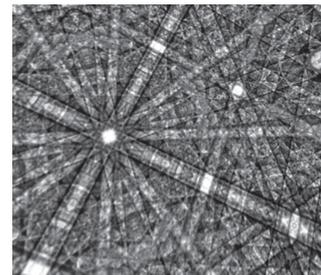
The detailed fine structure in the patterns is accurately reproduced: Characteristic HOLZ rings are found around the prominent zone axes
