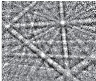
Experimental low pixel resolution patterns (160x120) acquired at high speed (7 ms), obtained with the eFlash EBSD detector
