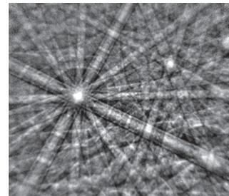
High resolution experimental Kikuchi pattern acquired with the eFlash EBSD detector
