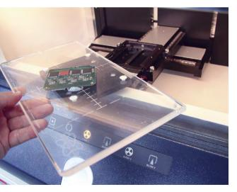
Standard quick-change stage interface Easy placement of a sample outside the sample chamber.
