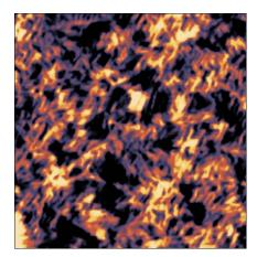
Fig 2: Topography image of crystalline polyethylene (z-range: 15 nm) measured at -120°C, scan size: 2  $\mu m$  x 2  $\mu m$
