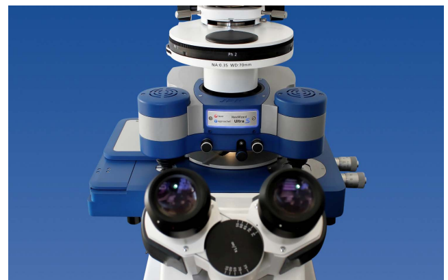
Figure 1. Typical setup of a NanoWizard® ULTRA Speed AFM on an inverted optical Zeiss microscope with motorised precision stage (20x20 mm 2 travel range). The AFM is further compatible with specific inverted models from Zeiss, Olympus, Nikon and Leica, commercial confocal microscopes, as well as TopViewOptics™ for opaque samples.
