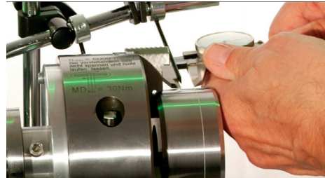
Figure 1c. Distance of string traveled is measured with verniers.
