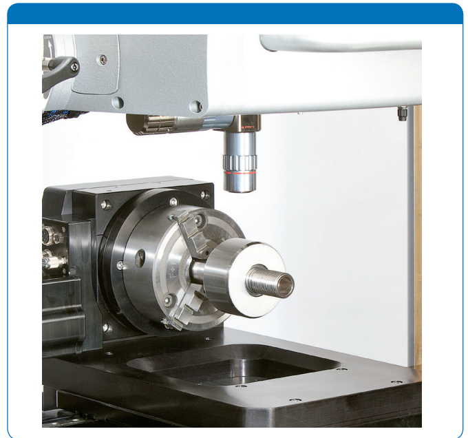
Figure 4. Test shaft mounted on NPFLEX-LA.
