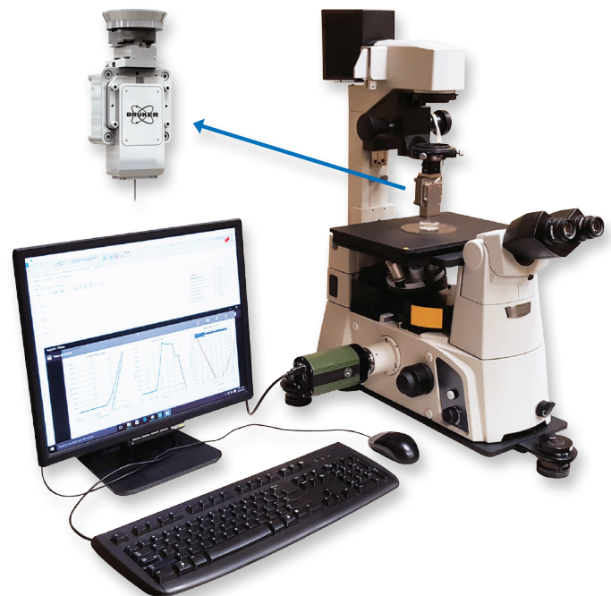
Figure 1. Hysitron BioSoft In-Situ Indenter performing testing while attached to an inverted optical microscope.
