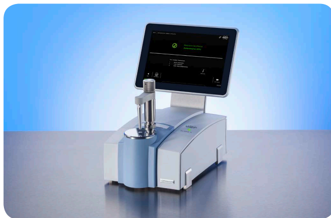
Figure 2: ALPHA II FTIR spectrometer equipped with the platinum diamond ATR and high pressure applicator.
