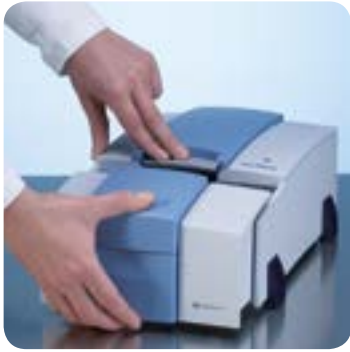
QuickSnap™ Sampling modules can easily be exchanged without the need for any tool.
