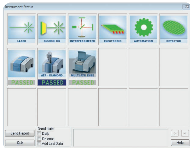
Fig. 3: Instrument Performance Guard showing the status of all spectrometer components and individual sampling modules.
