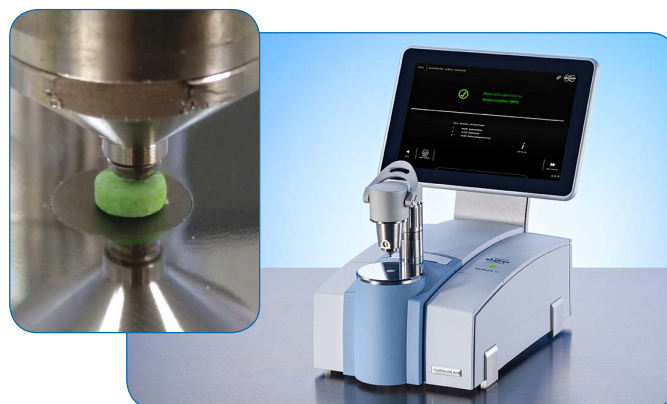
Figure 1: ALPHA II FTIR spectrometer with touch-PC (right). Samples are directly pressed onto the ATR crystal for analysis (left).
