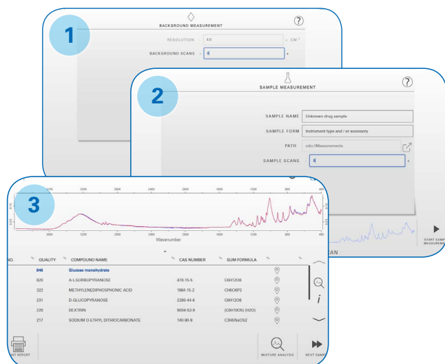
Figure 2: Easy as 1-2-3. Start with the background (1), take a quick look at the preview (2), and begin the analysis to get clear results in less than a minute (3).
