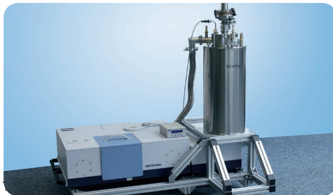
Fig. 8: Customized module for Silicon impurity photoluminescence, adapted to a VERTEX 80v FT-IR spectrometer. The samples are mounted in a liquid Helium bath cryostat in order to compensate the heat, created by the visible excitation laser
